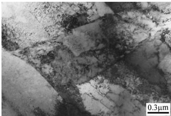
Figure 8 The electron microscopic contrast image of subgrains in the Fe-30%Ni alloy. The specimen was hold 3 s after deformation 20% at 1000°C, then quenched in water.
